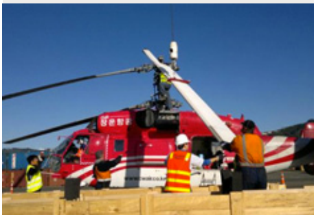
Wellington Port, New Zealand. The Kamov's huge blades are removed prior to being loaded onto the M.V. Pacific Resolution to Papua New Guinea. Photo: Sigit H Samsu, BMS.
